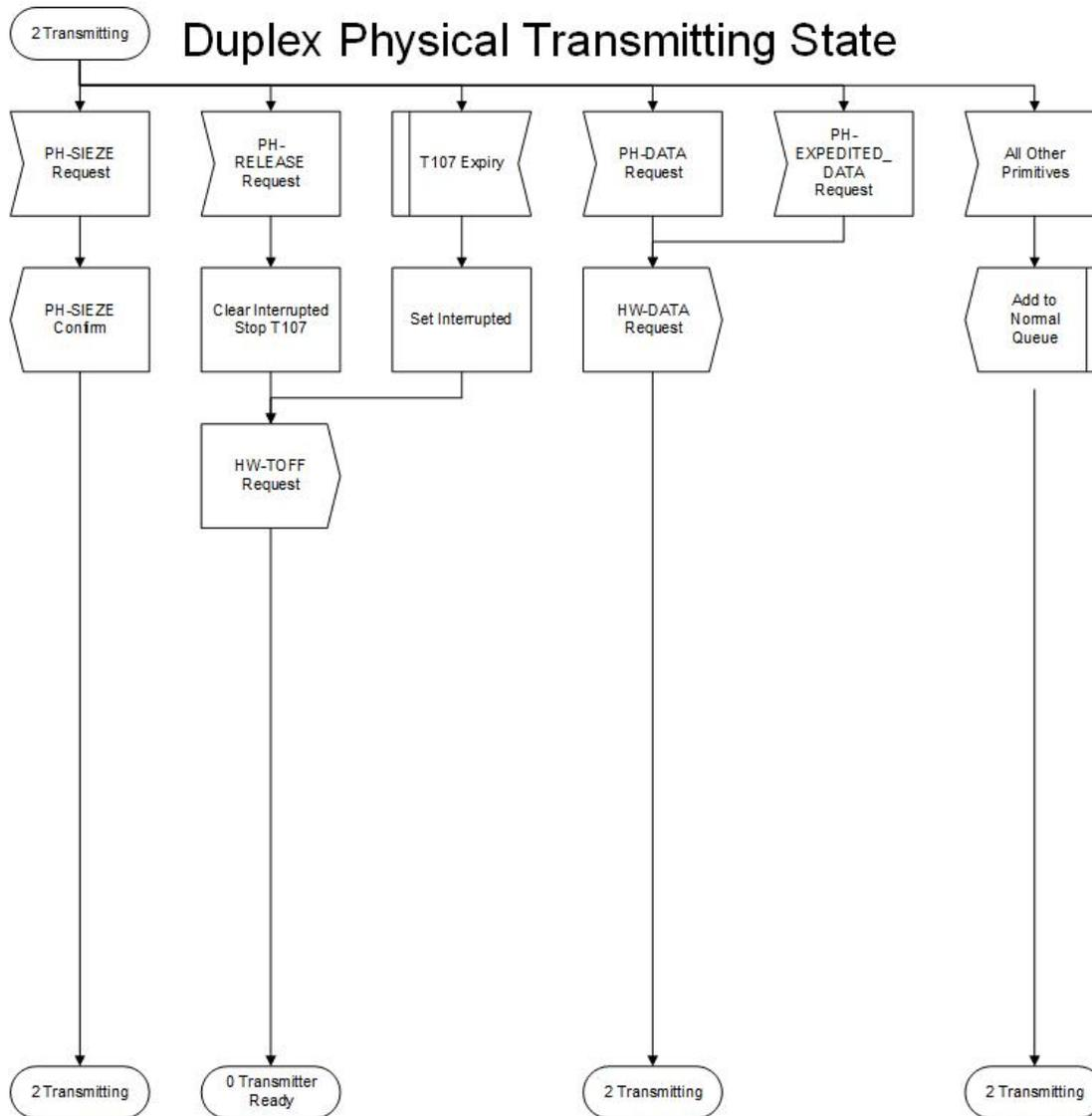
**Figure C2b.5 Duplex Physical Transmitting State.**
