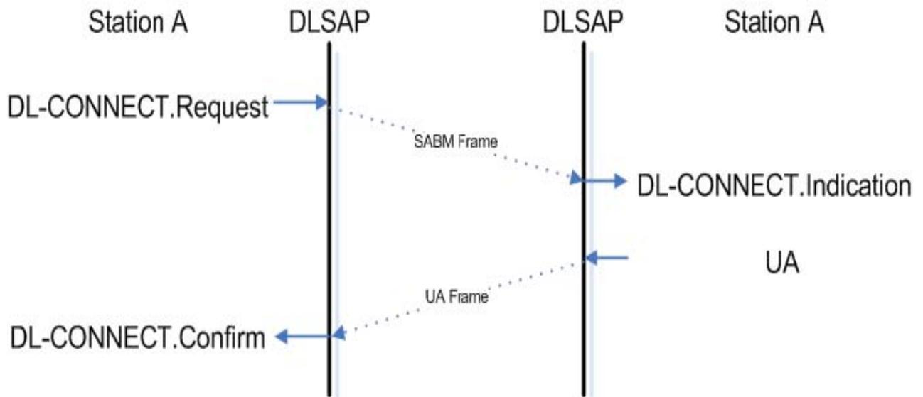
**Figure 2.4 Example Use Of AX.25 Primitive Types.**
