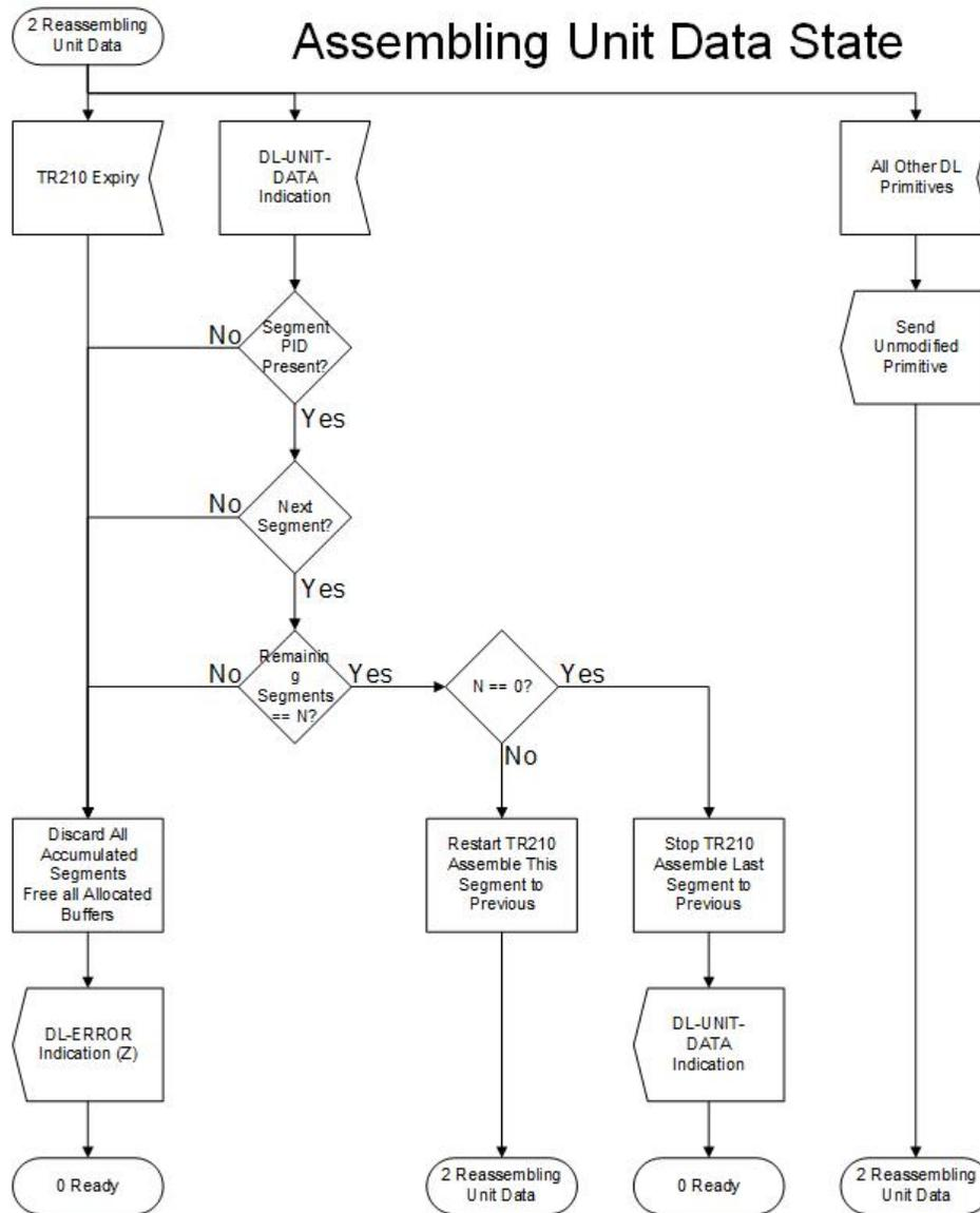
**Figure C-6.4 Reassembler Assembling Unit Data State.**
