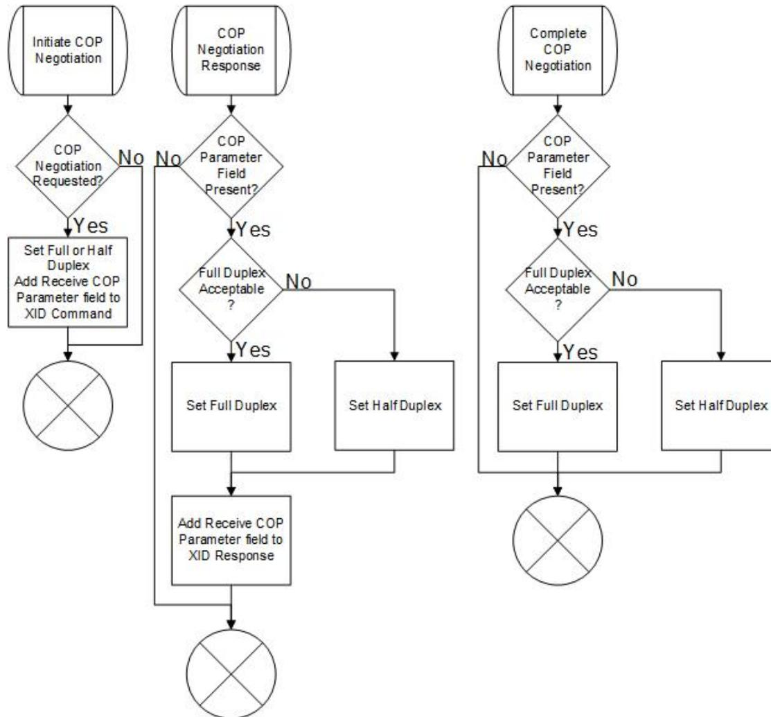
Figure C5.3 MDL Classes of Procedures Negotiation Subroutines.
