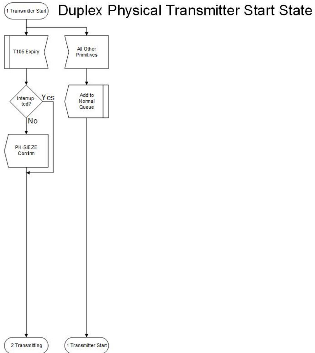
**Figure C2b.4 Duplex Physical Transmitter Start State.**
