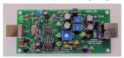
timed radio PTT keying. This USB sound card provides flat response, wide bandwidth audio, and manual audio level adjustments for transmit and receive along with software controlled non-relay transmitter PTT keying. To reach full performance with VARA FM or 9600 baud AX.25 packet it is necessary to use the higher baud rates and
