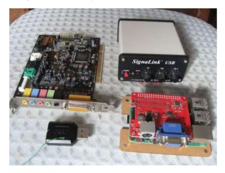
Starting in the upper left is an old "sound card" that plugged into the motherboard.
