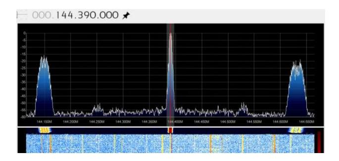
The side lobes seem to be an artifact from the SDR receiver, not a dirty transmitter. The same thing is seen with a much different transmitter.
