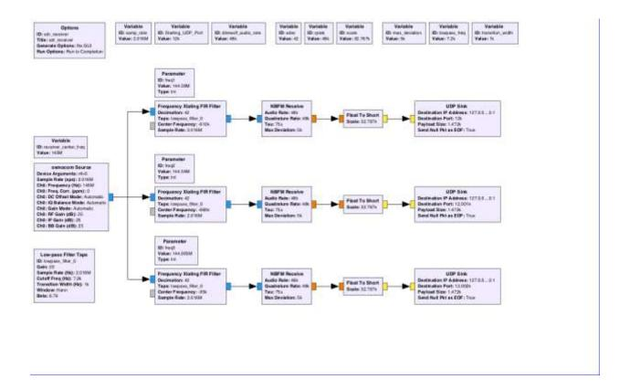
What I've routinely done is to use GnuRadio (ultimately a python script) for listening to multiple frequencies with a single SDR dongle (assuming they're all within ~2.4MHz of each
